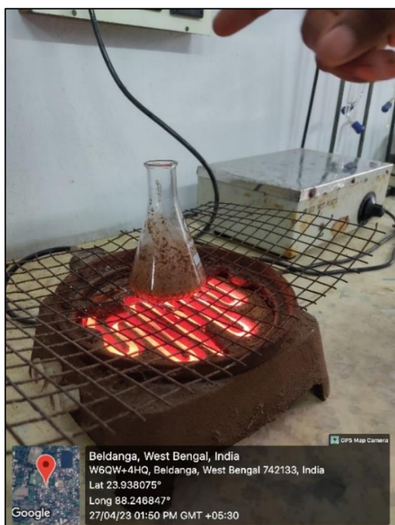
Fig 33 & Fig 34: Determination of phosphate in soil sample
