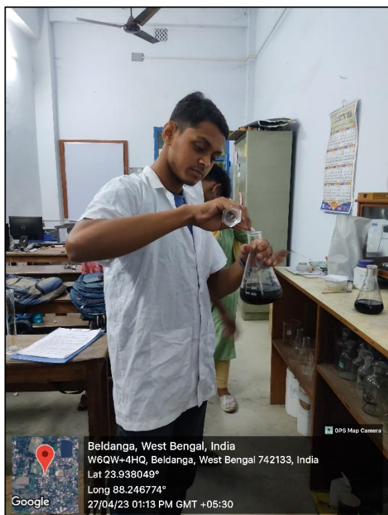
Fig 45 & Fig 46: Determination of Organic Carbon in soil sample
