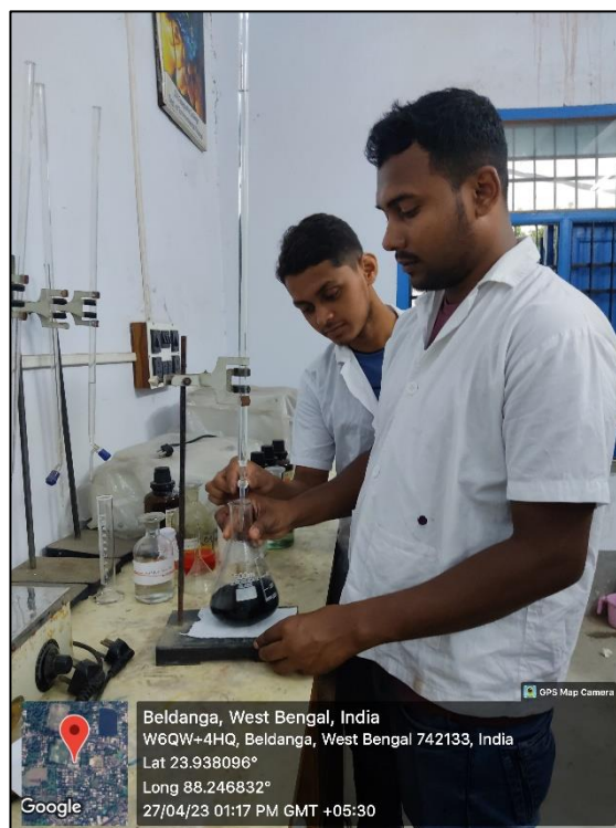
Fig 45 & Fig 46: Determination of Organic Carbon in soil sample
