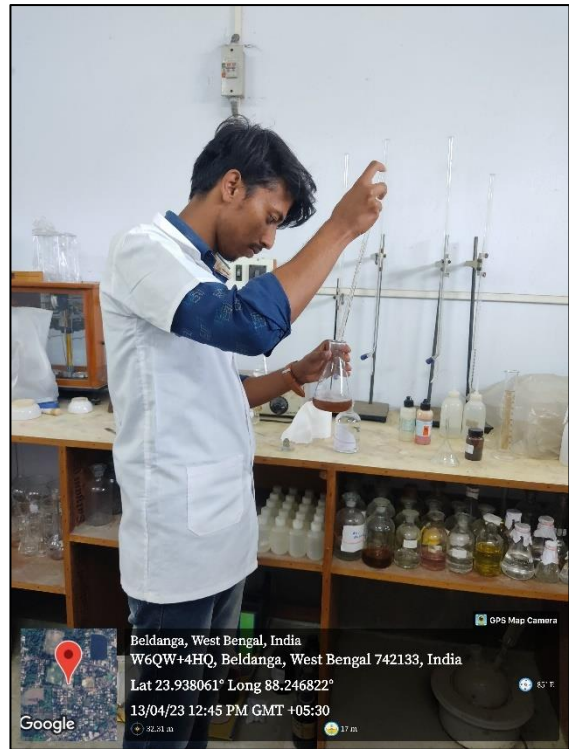
Fig 15 & Fig 16: Determination of alkalinity in water sample
