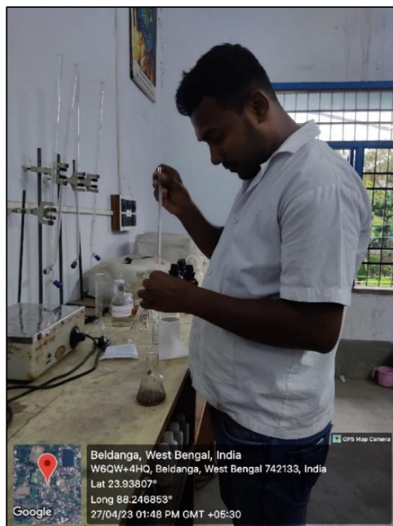
Fig 31 & Fig 32: Determination of phosphate in soil sample
